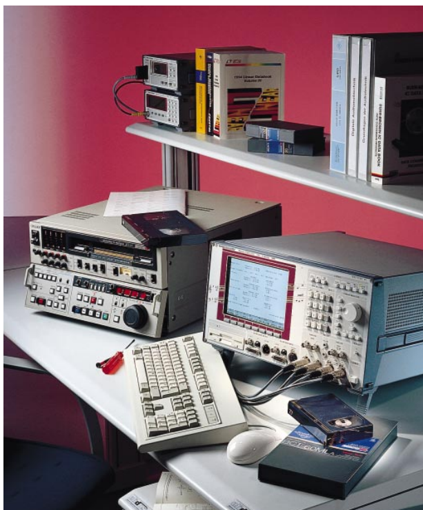
FIG 1 Automatic measurement on tape recorder with Audio Analyzer UPD Photo 42 400/2
