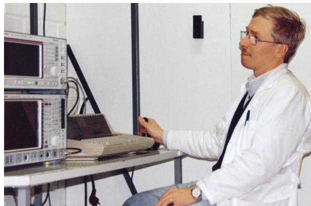
FIG 1 High-quality test setup comprising Signal Generator SMT and Spectrum Analyzer FSEA used for measuring antenna radiation patterns Photo: Huurrekorpi
